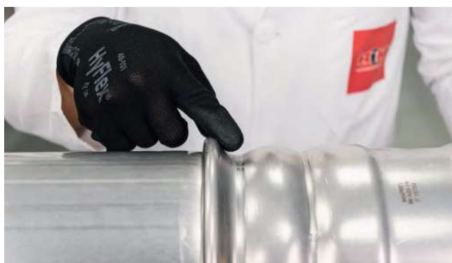
Figure 36 – Visual inspection of oversize pressing
