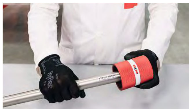
Figure 26 - Deburring the pipe
