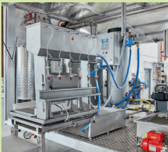
Extendable bottle and/or Bag-in-Box filler for comfortable operation.
