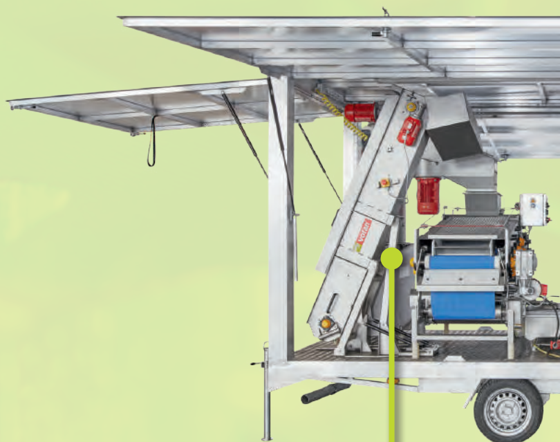
Fold-out elevator with charging hopper
